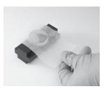
Slowly pull the lens paper across the lens so the cleaning fluid comes in contact with the entire lens surface. Finish pulling the paper across so all of the fluid has dried from the lens.
